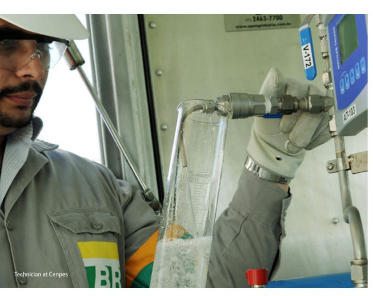
It gathers, in an integrated way, the instruments that are responsible for acquisition of analytical data related to water quality monitoring in cooling systems. It was built in habitable container structure, in order to allow it to move to the operational units.
