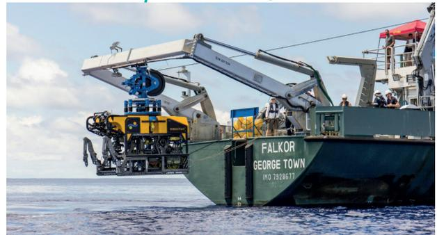
Fonte: 4500 m Remotely Operated Vehicle (ROV) - Schmidt Ocean Institute
